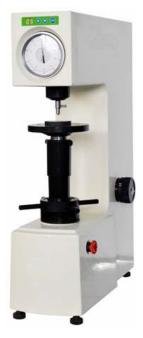
VEXUS SHR-150E Motorized Rockwell hardness tester adopts the mechanism of automatic loading and unloading of the test force, the test force is regulated by the load-change hand wheel. It can select the dwell time and is very easy to use. Besides setting zero to dial, there is no man-made error. The instrument has high sensitivity and stability.
