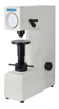
VEXUS SHR-150M Rockwell hardness tester is a popular-used hardness testing instrument to measure the hardness of the metal materials. No need power supply, the speed of the test force loading is regulated by the buffer and the test force is regulated by the load-change hand wheel. It has easy operation and stable performance, therefore it is widely used.
